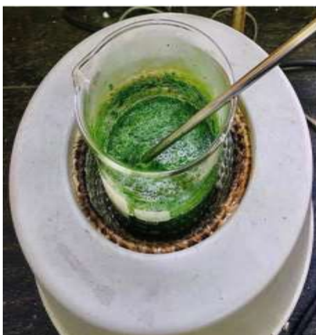
The mixture of Alumina nitrate and C. Papaya leave was heated at 70°C for 30 min in a Heating Mantle
